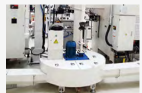
Centralized coolant system
