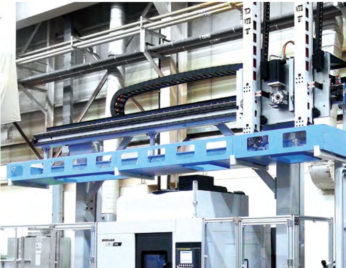
Gantry loader system
