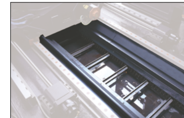
Center through Chip disposal
